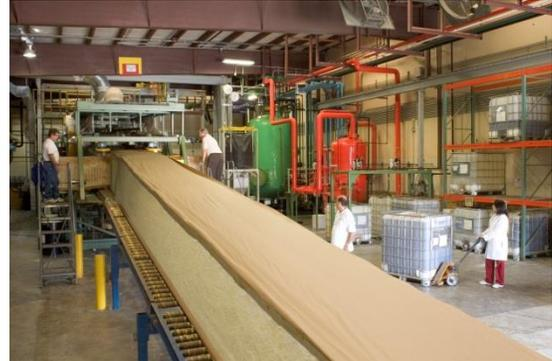
Figure 8: Polyiso exiting the tunnel
